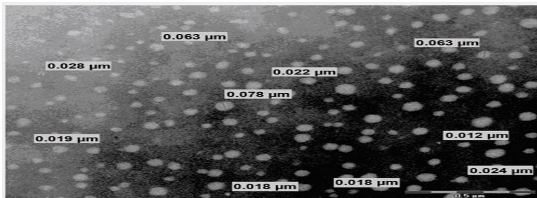
**Figure 2.** Transmission electron microscopic positive image of aceclofenac nanoemulsion showing the size of some oil droplets.
