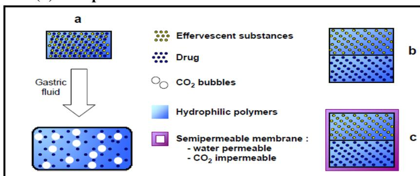
Figure 4: Schematic representation of “floating pill” proposed by Ichikawa (a). The penetration of water into effervescent layer leads to a CO<sub>2</sub> generation and makes the system float (b).
