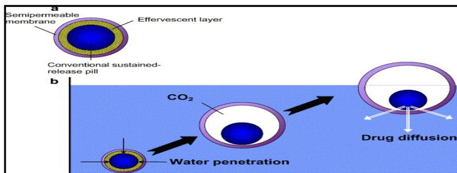
Figure 5: Schematic presentation of the structure of the floating matrix tablets
