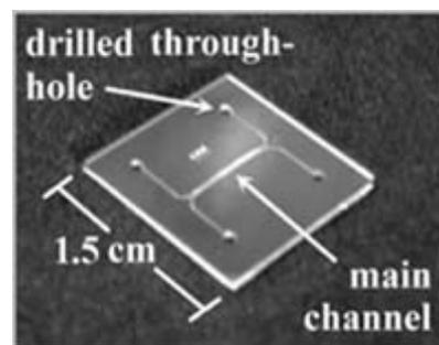
**Figure 1: Photographic image of Si-Pyrex microdevice**
