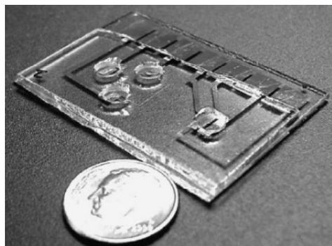
Figure 2: Photograph of a glass CE/EC microchip with integrated electrochemical detection and high voltage electrodes
